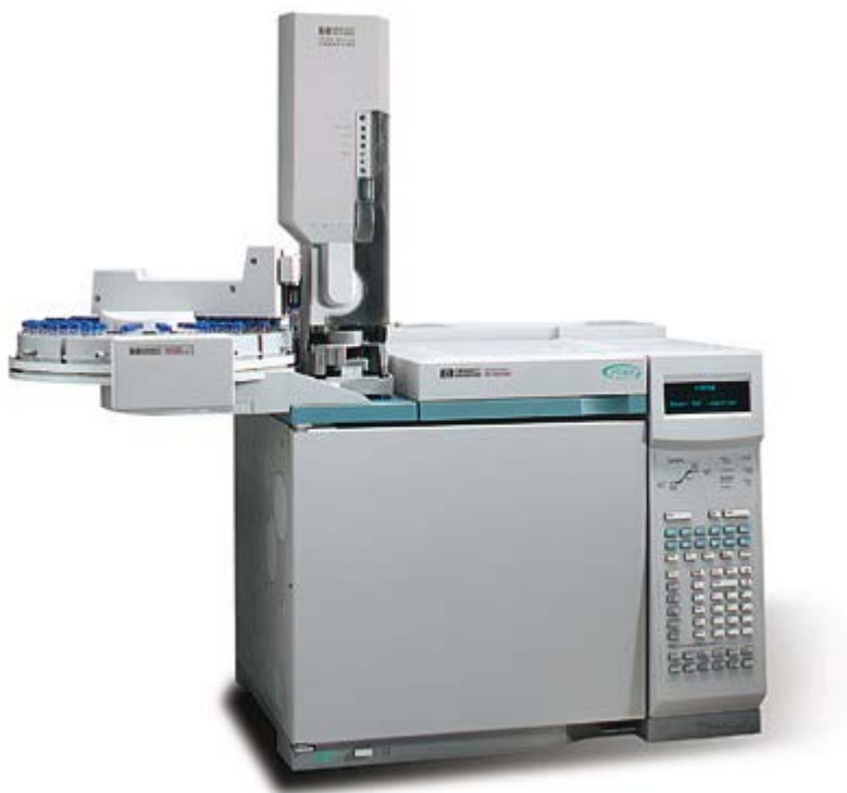
Labmax gas chromatograph machine which is used to measure VOC
